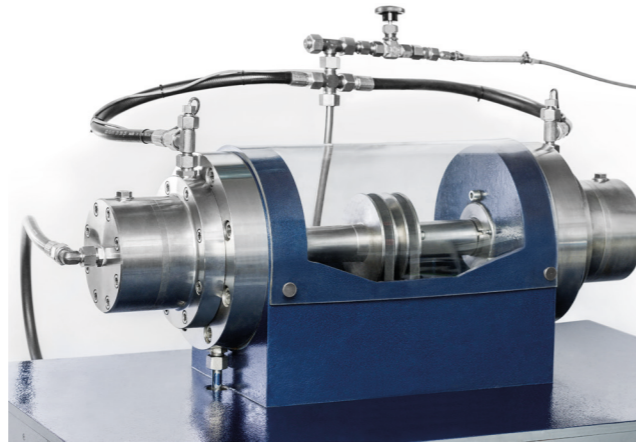
Figure 2: High-pressure face seal test rig
