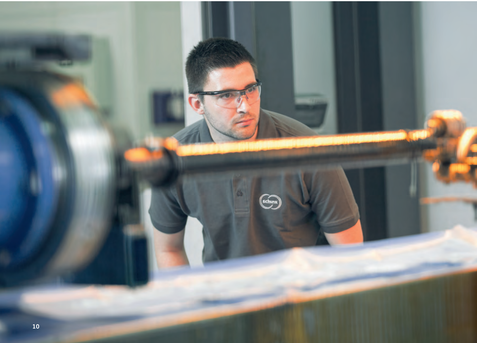
Filament winding for C/C and CFRP components
