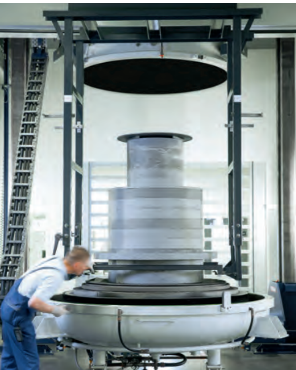
CVD-PyC coating under cleanroom conditions
