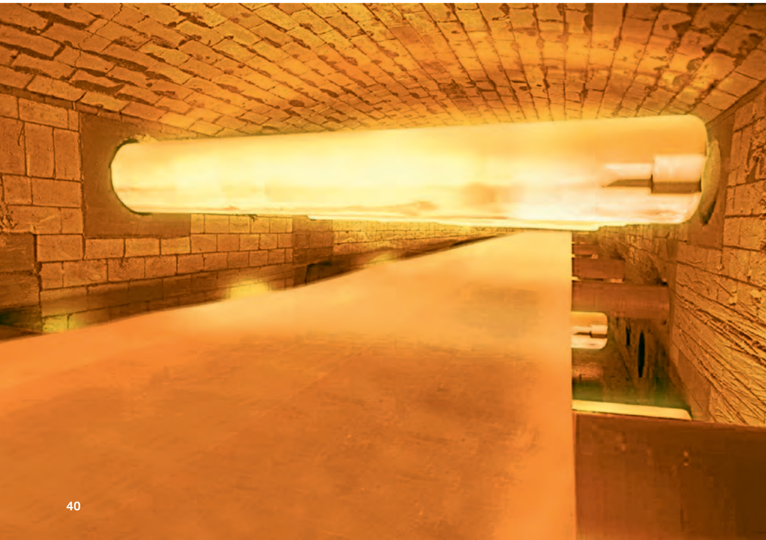
SiSiC radiant tubes in continuous annealing line
