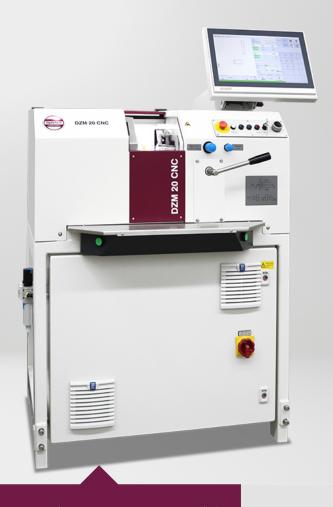
The DZM 20 CNC is a compact and easy to operate CNC controlled centering machine especially suited for super micro-optics and endoscopes. Clamping of the lenses using clamping bells or HD 12 runners.
