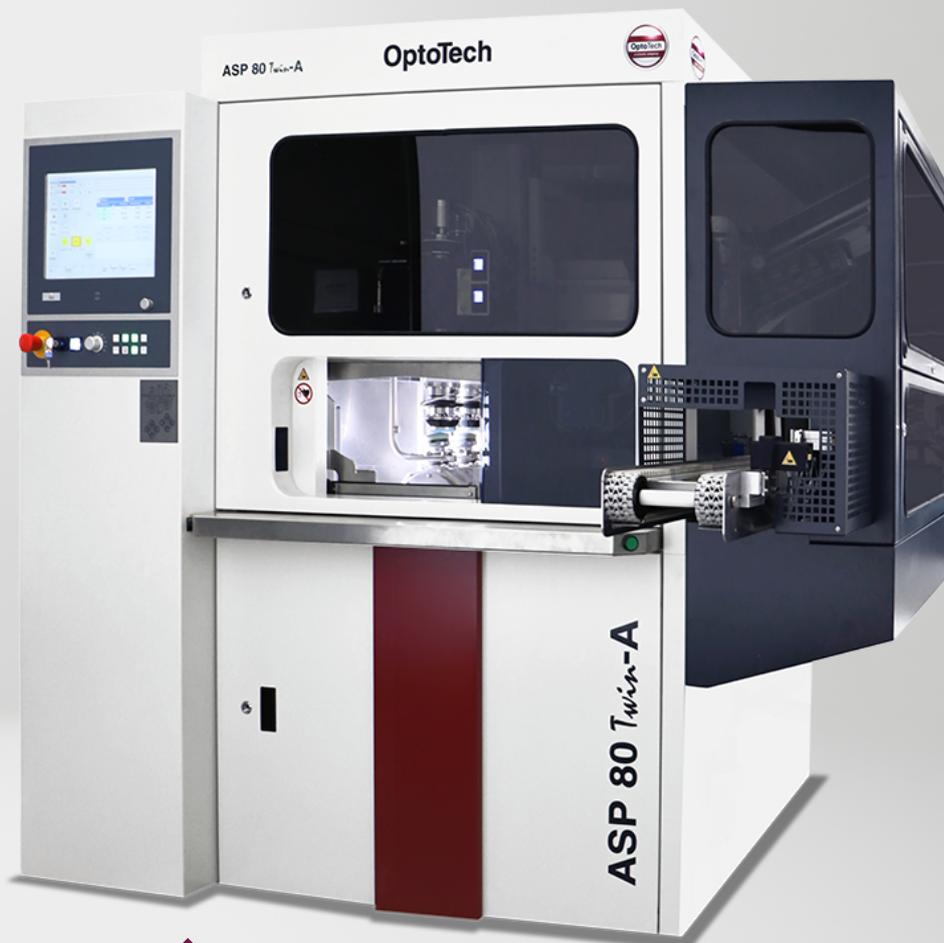
The OptoTech Digital-Surfacing-Polisher ASP 80 Twin-A is designed for full automatic high speed polishing of two toric/atoric or backside progressive lenses simultaneously. Round, oval, or lenses of any other shape can be polished.
