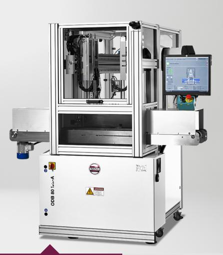
The OptoTech auto de-blocker ODB 80 Twin-A is designed for professional fully automated alloy deblocking. The machine allows uninterrupted de-blocking with no downtime.
