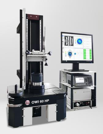
The compact Fizeau workshop interferometers OWI 60 HP and OWI 60 HP Invers are ideal tools for measuring of optical components. Several options allow the adaptation of these measuring devices to individual measuring tasks.
