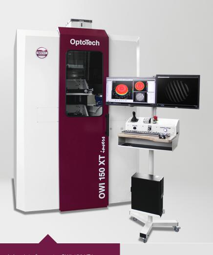
High precision Fizeau workshop interferometer OWI 150 XT invers for testing of spherical and aspherical surfaces. High precision kinematics and a working range up to Ø 150 mm make this measuring machine an indispensable tool for the production of high-end optics.
