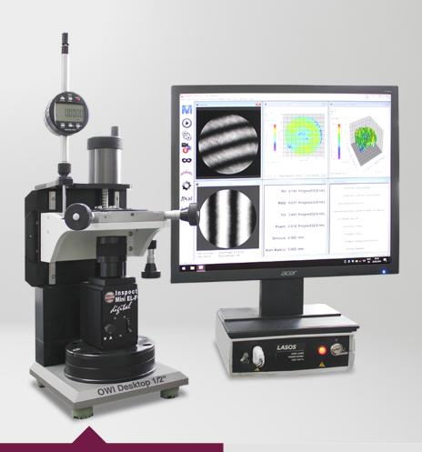
The compact workshop interferometer OWI Desktop 1/2" is the ideal measuring machine for endoscopy and micro production
