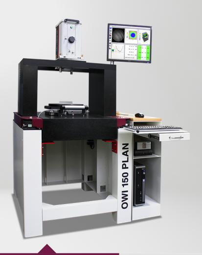
The workshop interferometer OWI 150 PLAN is the ideal measurement system for testing plano single surfaces or lenses produced as multi blocks.
