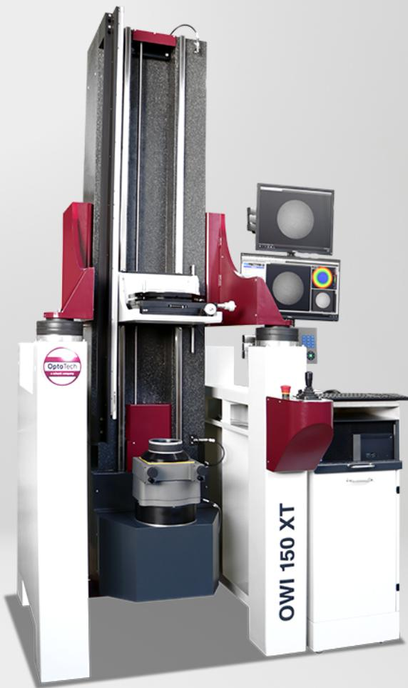
High precision Fizeau workshop interferometer OWI 150 XT 1500 for testing of spherical and aspherical surfaces. High precision kinematics and a working range up to  $\varnothing$  150 mm make this measuring machine an indispensable tool for the production of high-end optics.
