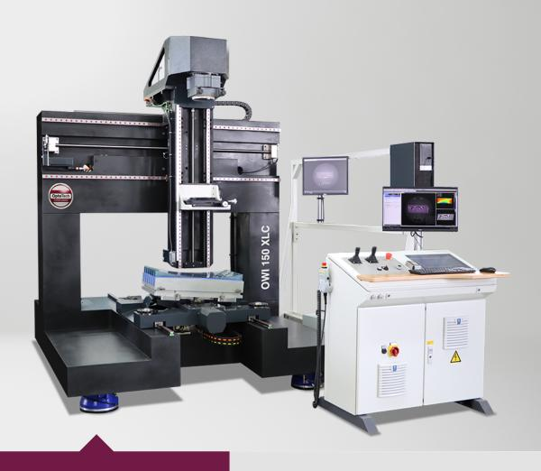
High precision Fizeau workshop interferometer OWI 150 XLC for testing of cylindrical and plano surfaces. Optimized kinematics and a large working range make this measuring machine an indispensable tool for the production of high-end optics.
