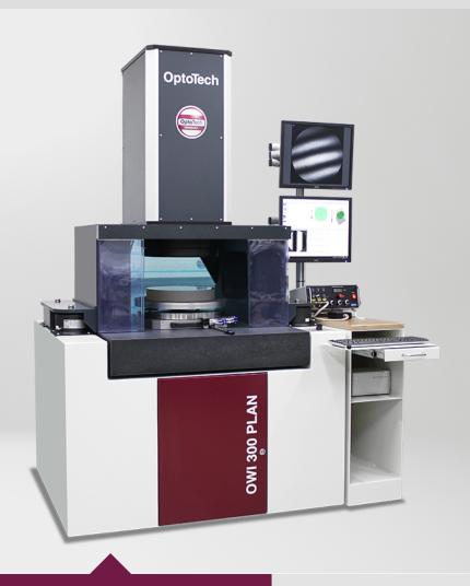
The workshop interferometer OWI 300 PLAN is the ideal measurement system for testing plano single surfaces or lenses produced as multi blocks.
