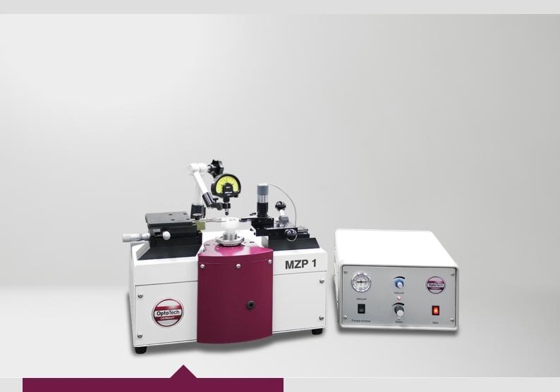
The mechanical centering testing unit MZP 1 excellently fits for easiest detection of centering errors of grinded optical components by using a measuring gauge.
