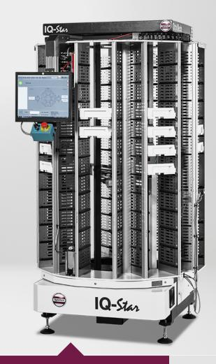
The OptoTech IQ-Star is the ideal solution for simple, low cost, space saving and intelligent LAB automation, which links the storage and distribution of job trays in an intelligent manner.
