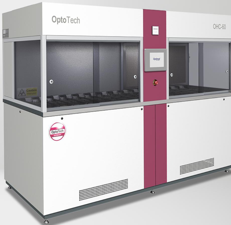
The OptoTech Hard Coating System (OHC) combines cleaning with ultrasonic and thermal cure dip coating for ophthalmic lenses. The OHC hardcoating systems are characterized by the product quality for which OptoTech is known, ease of use, and exceptional reliability in the daily production operation. Our hardcoating systems use well proven technologies to deliver pristine lens surfaces in superior quality.
