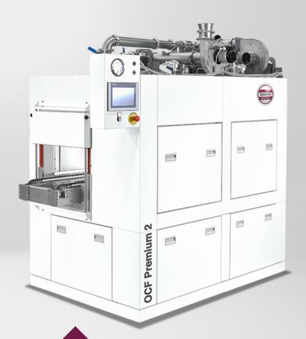
The OCF Premium 2 is especially designed for curing coatings on ophthalmic lenses in a continuous conveyor furnace after the hardcoating process. The modular system has 2 individually controlled heating zones whose working temperature can be set independently of each other offering maximum process flexibility.
