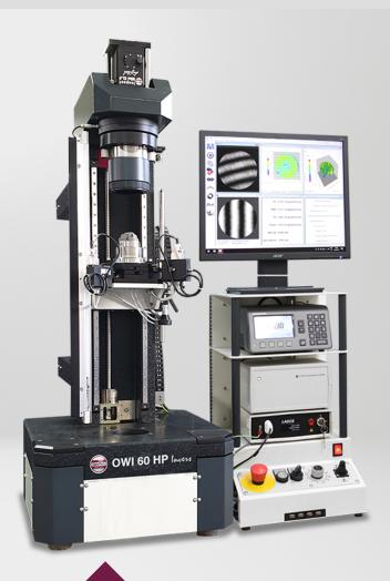
The compact Fizeau workshop interferometers OWI 60 HP and OWI 60 HP Invers are ideal tools for measuring of optical components. Several options allow the adaptation of these measuring devices to individual measuring tasks.
