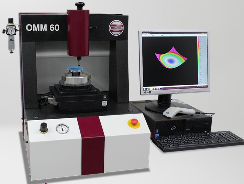
The new inexpensive freeform Measuring machine OMM 60 is an essential tool for quality inspection in freeform lens production. The OMM 60 is able to measure convex and concave lenses as well as grinded and polished surfaces.
