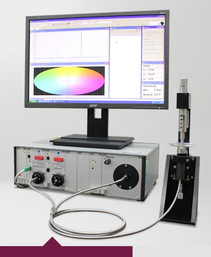
The OptoTech Spectrophotometer ETA-ARC is a fast, precise and easy-to-use measuring system for thin film coatings and hard coatings.
