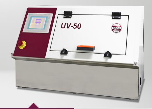
Quality test of the coating through accelerated aging under treatment with heat, humidity and UV-radiation.
