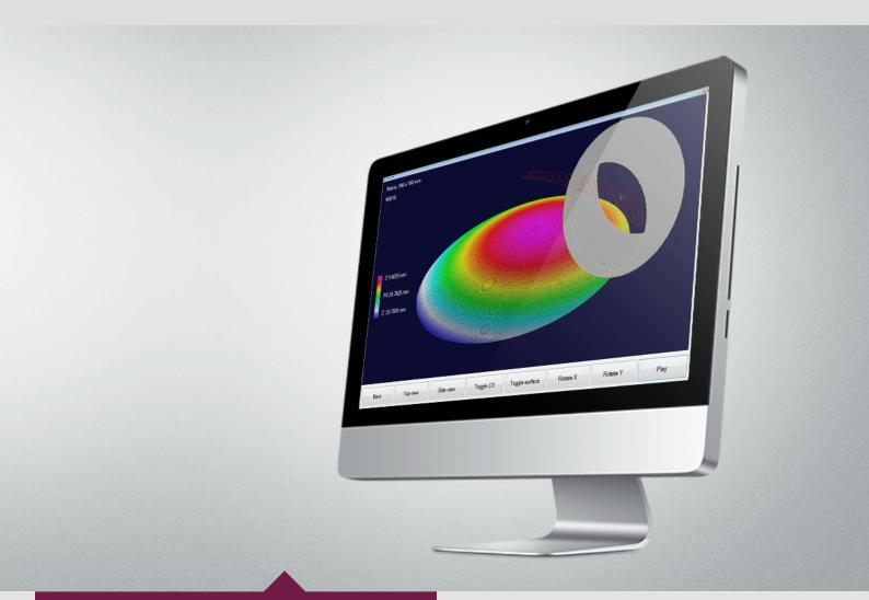
Software to create and manage files for the production of rotationally symmetric aspheres (2D mode), off-axis aspherical and toric surfaces, as well as freefrom surfaces (3D mode) depending on the machine type.
