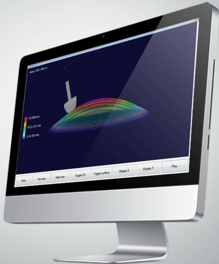
Software package for polishing and fine-correction of spherical and aspherical optics, plano and cylinder optics as well as freeform surfaces in 3D mode.
