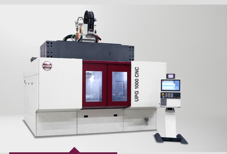
The Ultra-Precision Grinding Machine UPG 1000 CNC was especially designed for cut to polish complete processing of high-end ASTRO optics up to diameter 1000 mm. Whether spheres, aspheres, or freeform surfaces, the UPG 1000 CNC offers highest precision grinding (all axes mounted hydrostatically). This compact and high efficient design allows an optimal production of all important future parts in the area of ASTRO-Optics, EUV-Optics and aerospace technology.
