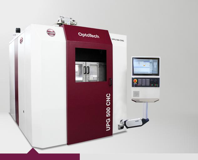
The Ultra-Precision Grinding Machine UPG 500 CNC was especially designed for processing of high-end optics up to diameter 500 mm. Whether spheres, aspheres, or freeform surfaces, the UPG 500 CNC offers highest precision grinding (all axes mounted hydrostatically).
