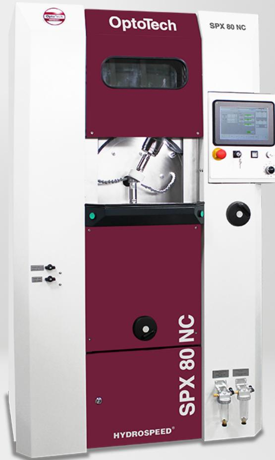
The OptoTech polishing machine SPX 80 NC is an ideal polisher for low as well as high aperture optics up to diameter 80 mm. The simple and efficient kinematics of this machine assures highest quality.
