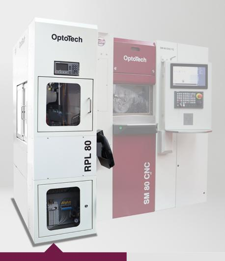
The RPL 80 is the high performance robot solution from OptoTech, that allows automatic loading and unloading of the SM 80 CNC-TC generator, the SPK 80 CNC polisher as well as the OWI 60 HP Invers-A interferometer. The RPL 80 can handle single surfaces (up to Ø80mm) as well as lenses on cementing pieces.
