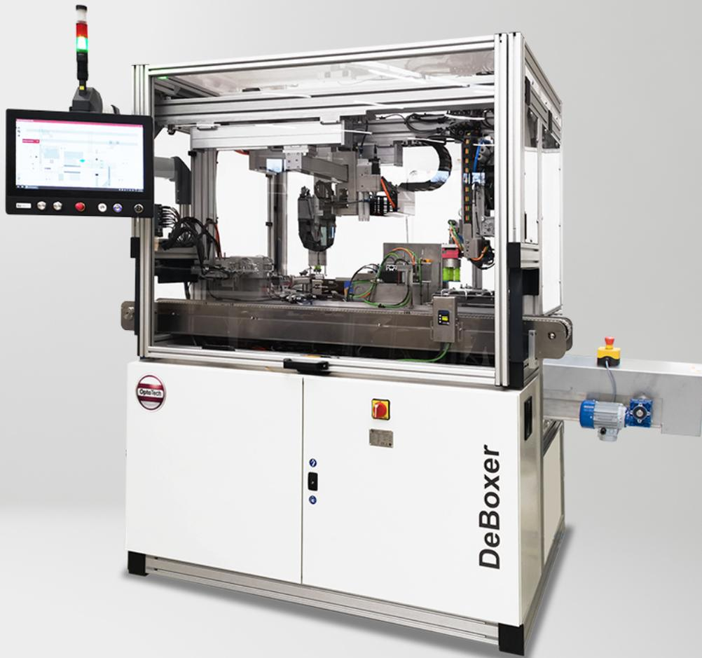
The new automatic DeBoxer is the first ever fully automatic system to specifically unpack semi-finished lenses. Depending on the type of boxes, this machine can unpack up to 300 lenses/h. Moreover, the DeBoxer can optionally be equipped with 2 outgoing conveyors for direct waste separation in carton and plastic.
