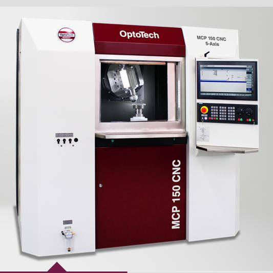
The new compact optical polishing centre MCP 150 CNC 5-Axis is one of the latest processing centres made by OptoTech.
