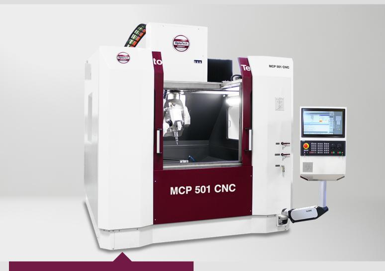
The multi-functional 6-Axis-Polishing Center MCP 501 CNC is an optimal machine for 3D production of any optical components. Whatever you want to produce, whether spheres or aspheres, the MCP 501 CNC is the perfect machine for these tasks. Multiple CNC axes and an innovative tool concept grant the requested flexibility.
