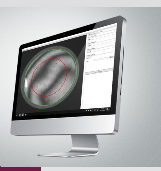
The visualization software  $\mu$ View is an essential tool for quality control in optical workshops and testing labs. It is designed for intuitive operation, ensuring the safe and efficient use of your measuring device. The interferometer image enables a quick initial inspection and precise evaluation of the test specimen.
