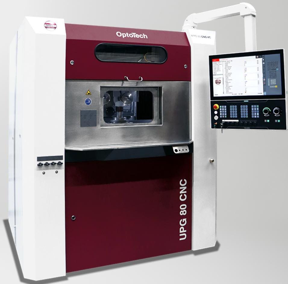
The UPG 80 CNC-2C is ideal for fine and ultra-precision grinding of optical surfaces and brittle-hard materials. With minimal subsurface damage, it significantly reduces polishing effort and time while ensuring excellent form accuracy. Precise axis guidance, a vibration-dampened design, and high-quality spindle bearings guarantee outstanding surface form and quality. Typical applications include semiconductor, SiC processing, aerospace, laser optics, and precision optics.
