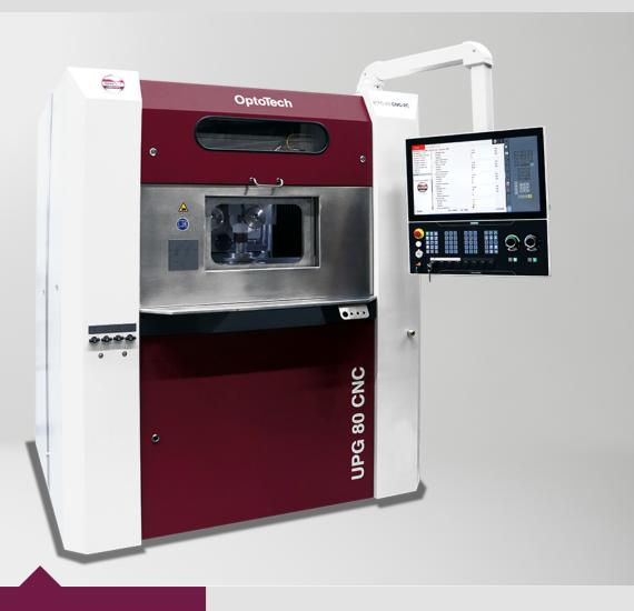
The UPG 80 CNC-2C is ideal for fine and ultra-precision grinding of optical surfaces and brittle-hard materials. With minimal subsurface damage, it significantly reduces polishing effort and time while ensuring excellent form accuracy. Precise axis guidance, a vibration-dampened design, and high-quality spindle bearings guarantee outstanding surface form and quality. Typical applications include semiconductor, SiC processing, aerospace, laser optics, and precision optics.
